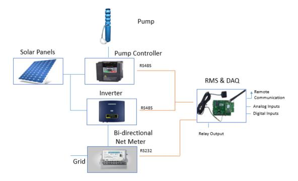
System Components and Architecture: PM KUSUM Component C or A: Option 3 (Solarisation of agricultural feeder at sub-station level)
